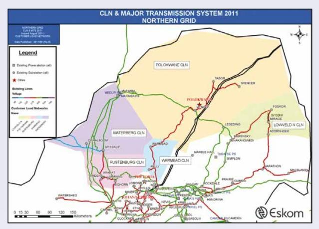
Figure 6.5: Current North Grid network and CLNs
