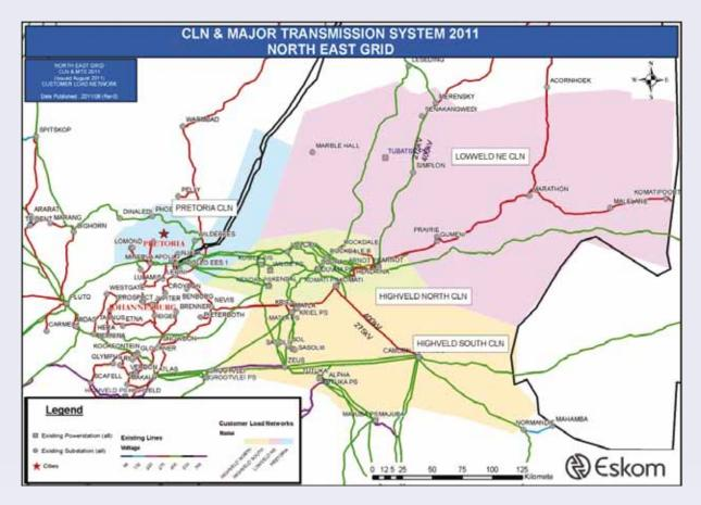
Figure 6.7: Current North East Grid network and CLNs
