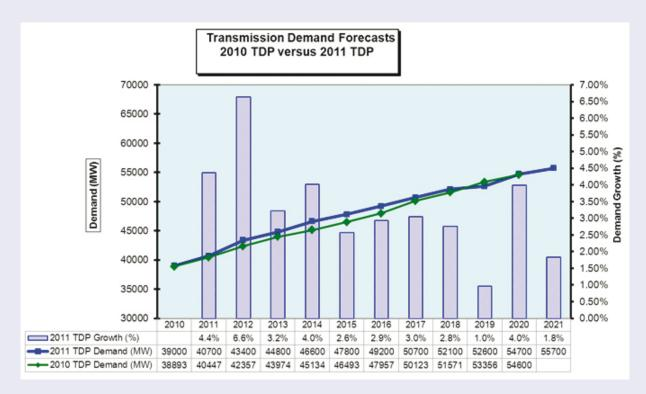
Figure 2.1: The Eskom Transmission System Demand Forecast
