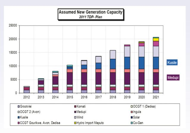
Figure 2.2: Power station capacity introduction by year
